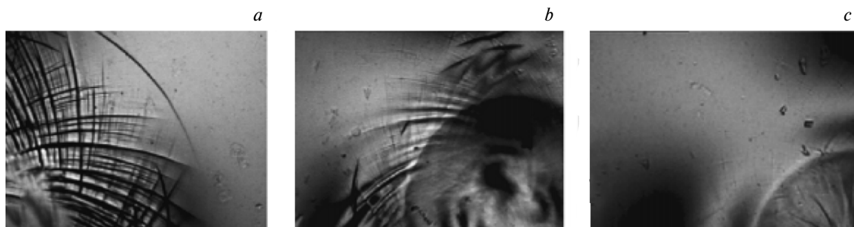
Fig. 18. Optical micrographs of the PET sample with shear bands after annealing at 40 ( a ), 70 ( b ), and 75 °C ( c ). 81
