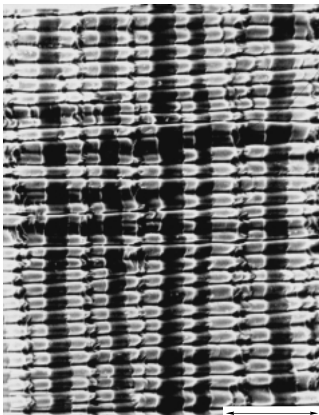
Fig. 2. Scanning electron micrograph of a polyethylene terephthalate specimen with a 4-nm-thick platinum coating after stretching at 100°C at a rate of 0.1 mm/min by 100% and subsequent additional stretching by 50% at higher stress.
