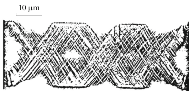
Fig. 5. Optical micrograph taken from a thin section of PS sample subjected to uniaxial compression along the vertical axis [35].
